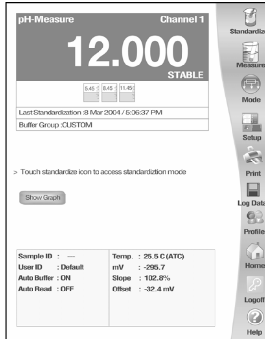
Once meter is calibrated, pH Measure screen shows standardized buffers and last standardization time/date
